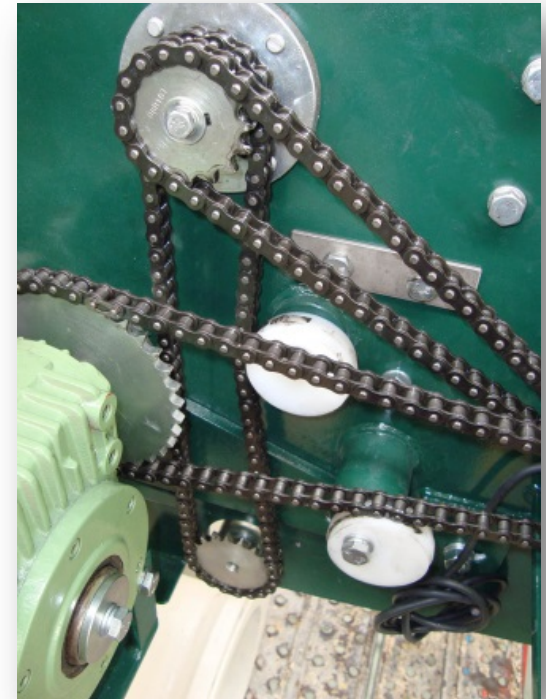
Chain system within a magnetic separator
